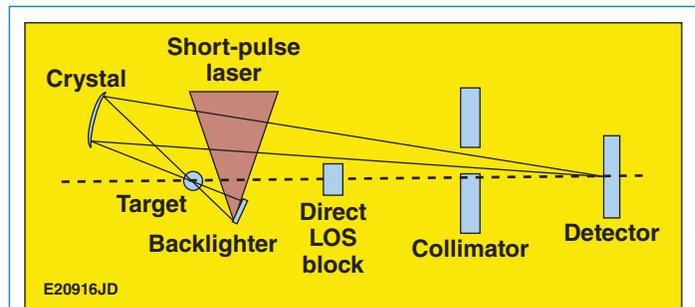
Figure 1. Schematic of the spherical crystal imager backlighting setup (not to scale). The short-pulse laser illuminates a backlighter foil behind the primary target, which is illuminated by 60 beams from the OMEGA laser (not shown). A direct line-of-sight (LOS) block and a collimator protect the detector from background x rays emitted by the backlighter and primary targets.
