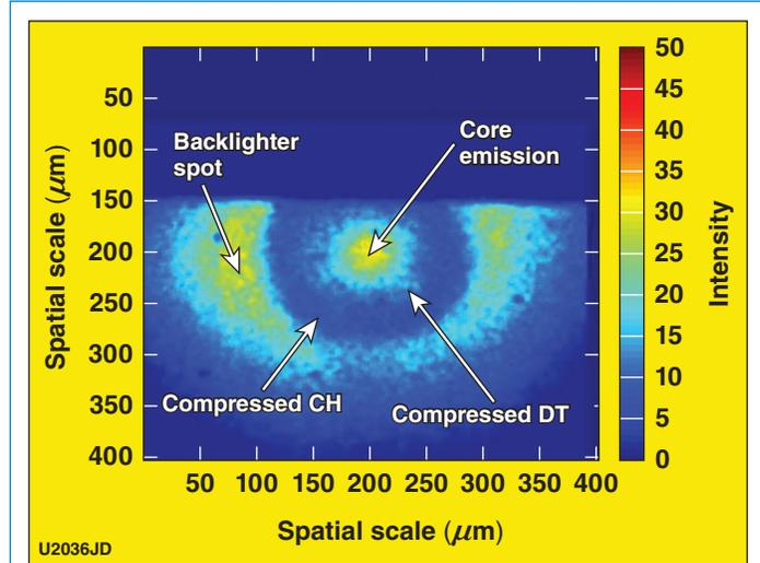
Figure 2. Radiograph of a cryogenic implosion recorded with the aberration-corrected narrowband crystal imager on a 40-ps exposure time framing camera at a convergence ratio CR  $\sim 7$ . The Si backlighter target was driven by a 20-ps, 1.5-kJ pulse from OMEGA EP. The image is rendered on a linear intensity scale.
