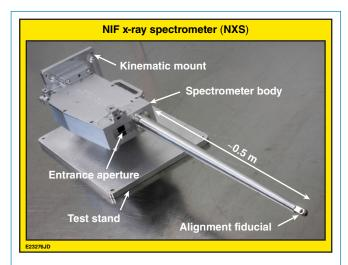
Figure 1. A photograph of one of the three NXS snouts delivered to the NIF. The NXS is secured to the DISC using a kinematic mount. The alignment fiducial guides the positioning of the NXS and DISC combination in the NIF target chamber with the diagnostic insertion manipulator.
