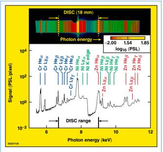
Figure 2. Calibration data recorded on OMEGA with NXS crystal pack #7 on an image-plate detector positioned in the DISC x-ray photocathode plane. Prominent K-shell emission lines are identified in the lineout with the DISC photon-energy range indicated.
