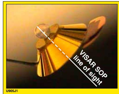
Figure 1. Photograph of a shock-timing target with a 950- $\mu\text{m}$ -diam, 100- $\mu\text{m}$ -thick CH shell. Cones are attached to shield the diagnostics from the drive laser.
