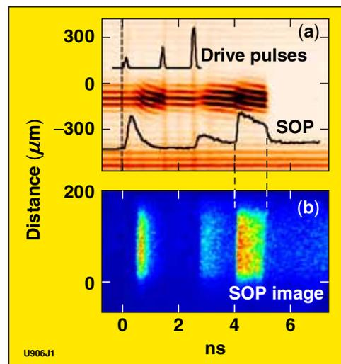
Figure 2. (a) The VISAR image for shot 54183 with intensity plots of the drive pulses and the SOP intensity. (b) The SOP image exhibits the shock-coalescence features observed in VISAR.
