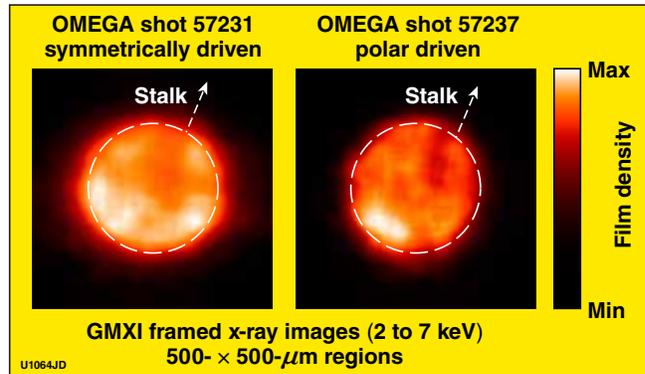
Figure 1. Film recorded framed x-ray images of the DT-filled glass-target implosion obtained with the GMXI near the time of stagnation ( $\sim 2.6$  ns after the start of the laser pulse), for both (a) a symmetrically driven target and (b) a polar-driven target. The target stalk direction is indicated by the dashed arrows.
