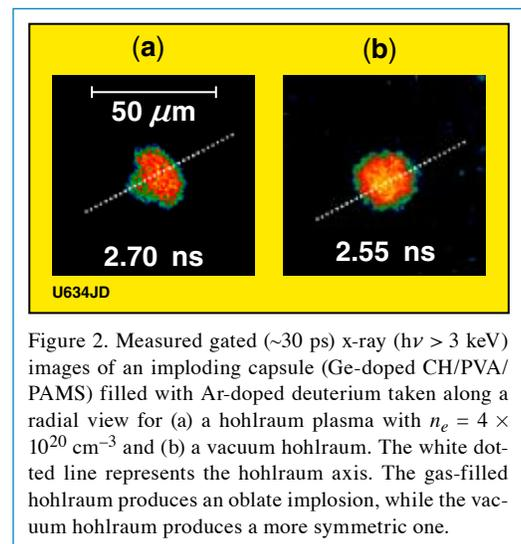
Figure 2. Measured gated ( $\sim 30$  ps) x-ray ( $h\nu > 3$  keV) images of an imploding capsule (Ge-doped CH/PVA/PAMS) filled with Ar-doped deuterium taken along a radial view for (a) a hohlraum plasma with  $n_e = 4 \times 10^{20} \text{ cm}^{-3}$  and (b) a vacuum hohlraum. The white dotted line represents the hohlraum axis. The gas-filled hohlraum produces an oblate implosion, while the vacuum hohlraum produces a more symmetric one.
