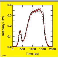
Figure 2. Pulse shape used to test the effect of a picket pulse added to the front of an  $\alpha = 5$  implosion pulse shape; specified pulse shape (blue solid line); actual pulse shape (red dots). The picket intensity is 40% of the peak intensity, and its peak precedes the time of the half-maximum intensity of the  $\alpha = 5$  pulse by 340 ps.
