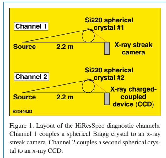
Figure 1. Layout of the HiResSpec diagnostic channels. Channel 1 couples a spherical Bragg crystal to an x-ray streak camera. Channel 2 couples a second spherical crystal to an x-ray CCD.
