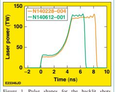
Figure 1. Pulse shapes for the backlit shots (N140612-001) compared to the previous shot (N140228-004) where only self-emission was used to infer trajectory.
