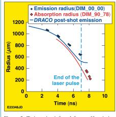
Figure 3. Trajectories inferred from self-emission images viewed from the pole compared to that inferred from backlit image viewed from the equator for NIF target shot N140612-001.
