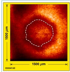
Figure 2. Images from backlit implosion N140612-001, using an Fe backlighter at a convergence ratio of ~2.8. The dashed line is the location of the surface of peak x-ray absorption.
