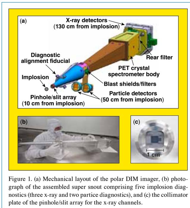
Figure 1. (a) Mechanical layout of the polar DIM imager, (b) photograph of the assembled super snout comprising five implosion diagnostics (three x-ray and two particle diagnostics), and (c) the collimator plate of the pinhole/slit array for the x-ray channels.
