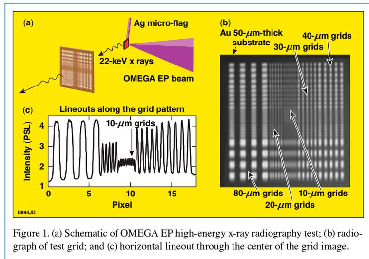
Figure 1. (a) Schematic of OMEGA EP high-energy x-ray radiography test; (b) radiograph of test grid; and (c) horizontal lineout through the center of the grid image.
