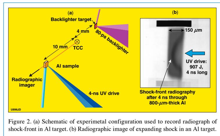
Figure 2. (a) Schematic of experimental configuration used to record radiograph of shock-front in Al target. (b) Radiographic image of expanding shock in an Al target.
