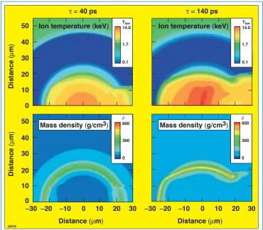
Figure 1. Ion-temperature and mass-density contours 40 ps and 140 ps after arrival of electron beams from *DRACO* simulation of fast-ignition capsule.
