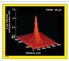
Figure 1. Enhancement of first x-ray image obtained on the OMEGA EP Laser System.
