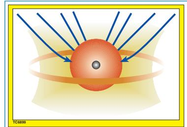
Figure 1. The Saturn target design for polar direct drive on the NIF uses the indirect-drive NIF ports with the beams re-pointed toward the equator and with a plastic ring placed around the target.
