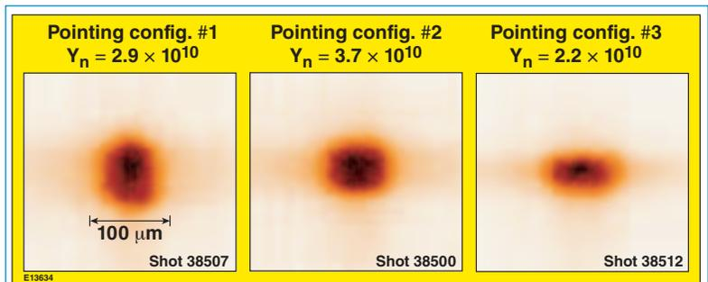
Figure 3. X-ray framing camera images of three Saturn targets irradiated with different beam-pointing configurations. Configuration #2 (center image), predicted to give optimum uniformity, produced the most symmetric core and the greatest neutron yield. The other configurations gave prolate and oblate cores, respectively, relative to the vertical axis and lower yields.
