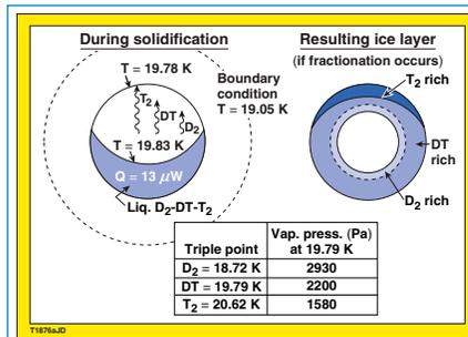
Figure 1. Schematic illustrating possible fractionation in a D<sub>2</sub>-DT-T<sub>2</sub> mixture within a cryogenic DT capsule. The triple point of the lighter molecules is lower than that of the heavier ones; this can lead to fractionation at slow rates of solidification.
