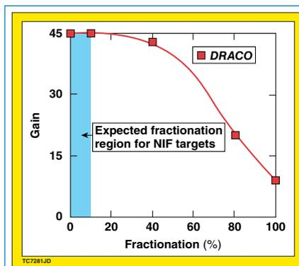
Figure 3. Calculated gain of a baseline direct-drive NIF capsule as a function of fractionation. For these simulations, the north polar region of the ice layer was assumed to be tritium rich.
