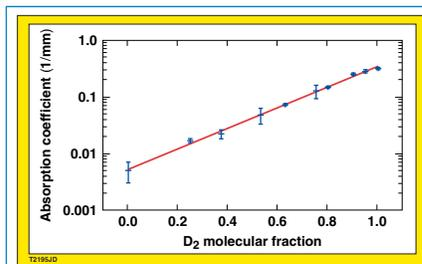
Figure 2. The measured average absorption coefficient of the D<sub>2</sub> in an HD mixture as a function of the D<sub>2</sub> molecular fraction at a wavelength of  $\lambda = 3.151 \mu\text{m}$ .
