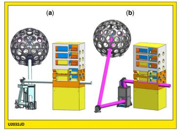
Figure 1. (a) Existing setup for bringing Beam 25 through port P9, with the beam detuned to  $2\omega$ . (b) Proposed setup for bringing Beam 35 through port P9. The beam remains at  $3\omega$ .
