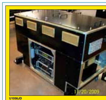
Figure 1. The NIF4 \omega Fidu laser system is built in a portable workstation in the NIF target bay so that it can be removed easily for high-yield target shots. The enclosure serves as both a laser safety barrier and provides EMI protection to the laser and electronics during target shots.
