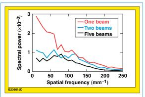
Figure 2. Power spectra of shock-velocity perturbations as a function of spatial frequency for three irradiation conditions: one, two, and five beams. As more beams are added, the drive uniformity increases and perturbations in shock velocity decrease.
