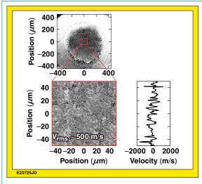
Figure 1. OMEGA high-resolution velocimeter (OHRV) interferometry data for a shock wave in a CH target driven by two OMEGA beams with 100-ps drive pulse. Modulations in image intensity are proportional to shock velocity. The insets show a magnification of the central 100- $\mu$ m square of the image and a lineout of that region.
