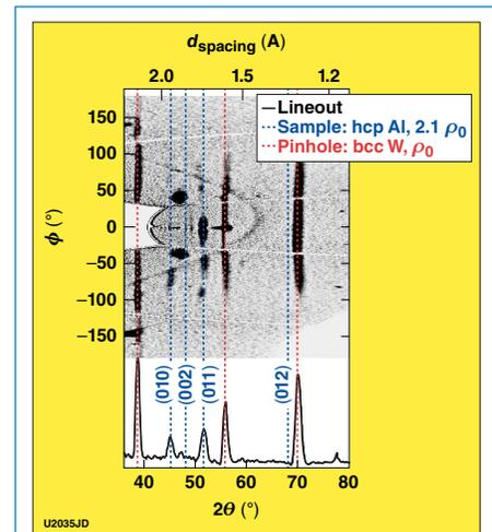
Figure 2. X-ray diffraction (XRD) image-plate data projected into  $2\theta$ – $\phi$  space for a shot at ~2.6 Mbar. The hcp aluminum diffraction lines at  $2.1 \rho_0$  are plotted in blue on top of the data. The lineout of the data at the bottom shows peaks in the pattern consistent with the hcp phase. Diffraction off of the bcc tungsten pinhole (shown in red) provides an *in-situ* calibration.
