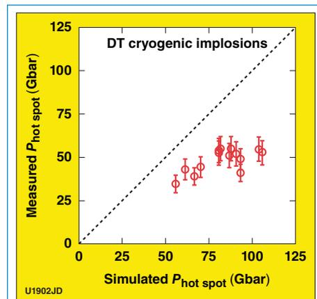
Figure 3. A comparison of the measured hot-spot pressure in DT cryogenic implosions with simulated values.
