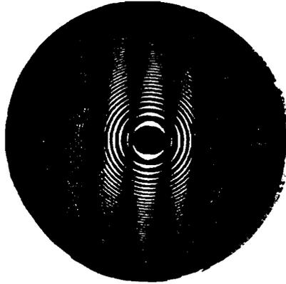
Figure 2.8 Moiré Pattern of Two Closely Spaced Overlapping Zone Plates
