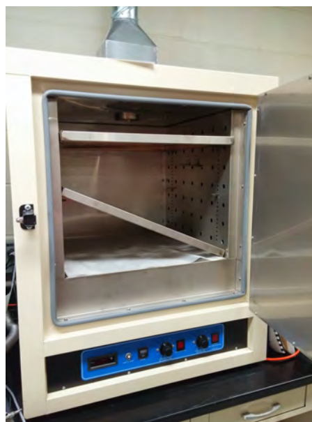
Figure 3.4: A VWR model 1350FD vacuum oven used for a variety of laboratory heating and drying applications.
