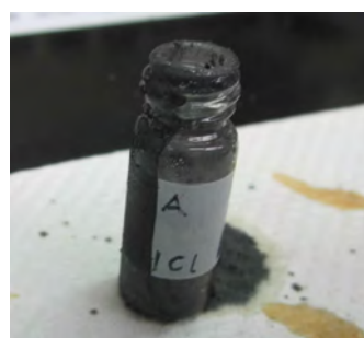
(e) Hydrochloric acid immediately corroded the HJR 5A sample, no others were tested.
