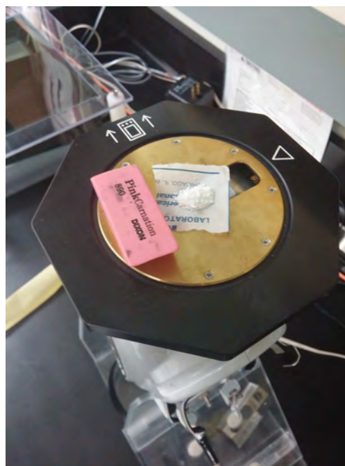
(d) Evaporated zirconium solution gel powder sample resting on wax-paper, ready for measurement. Eraser provided for scale.
