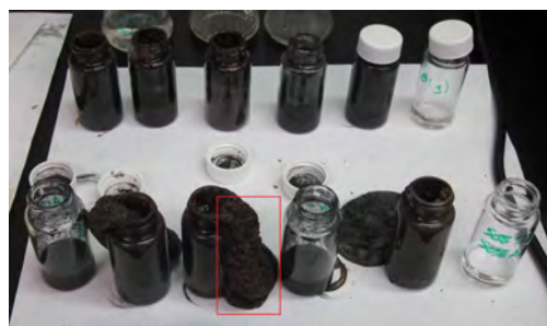
(b) MR powder dispersed in 100% acetic acid (top), and 50% acetic acid and 50% DI water (bottom). Foam produced during MR powder corrosion is highlighted.
