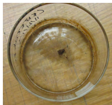
(e) The sediment isolated from the vials shown in Figure 5.3d was placed into a dish and then put in a vacuum oven, at 100°C, 525 – 675 Torr to evaporate the solution.
