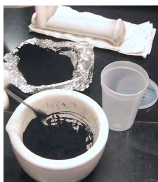
(g) Dried MRF powder that has been freshly milled, prepared to be transferred to a plastic cup for storage.
