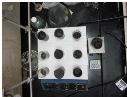
(b) Corrosion test of powder samples HJR 8B and 13B, 9:00 hours into the test. Six of the ten samples have corroded, as evidenced by the foam emitting from the beakers.
