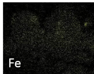
(b) An X-ray map showing the location and concentration of iron in Figure 6.21a
