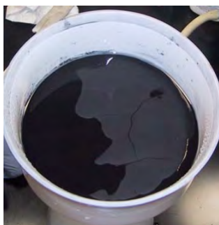
(d) Top view of the powder being vacuum dried prior to being placed into petri dishes and loaded into the oven.
