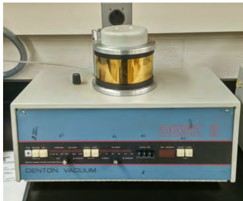
(a) Denton Desk II vacuum sputter coating instrument, used to gold sputter coat various samples for the SEM.
