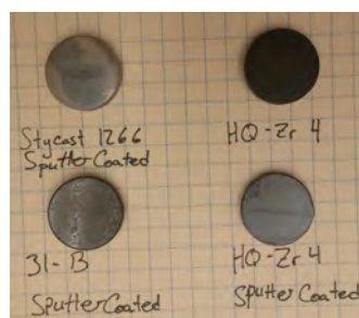
(b) Four polished epoxy pucks, from upper left to lower right: A sputter coated 'blank', HQ-Zr 4 in Stycast 1266 with no sputter coating, sputter coated 31-B, sputter coated HQ-Zr 4.
