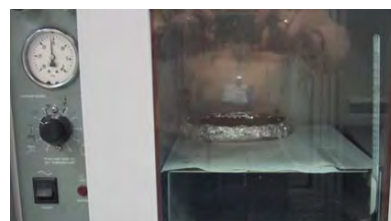
(f) Condensation accumulating on the interior of the vacuum oven after approximately one half hour of drying.
