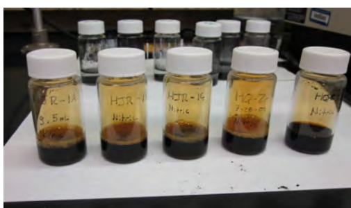
(a) 10 vol.% MR powder dispersed in: 68% nitric acid and 32% DI water
