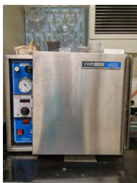
(e) A VWR model 1410D vacuum oven used for a variety of laboratory heating and drying applications.
