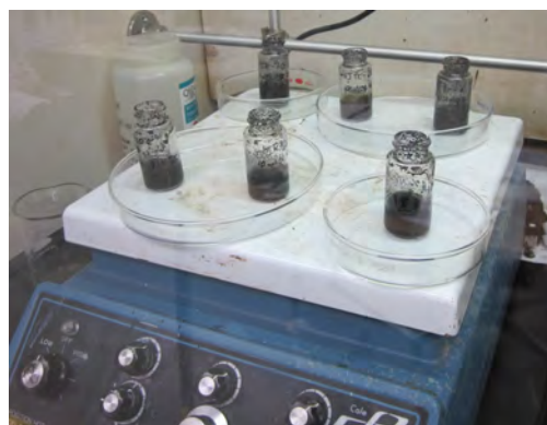
Figure 3.10: Dilute nitric acid corrosion test utilizing magnetic stir-bars and a 9 location stir-plate
