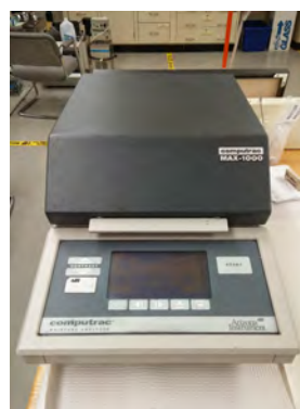
(h) An Arizona Instruments Computrac Max-1000 moisture content analyzer used to determine moisture content of various laboratory samples.
