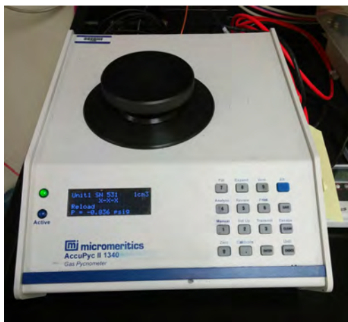
(a) Micromeritics Accupyc II 1350 helium gas pycnometer, used for powder density measurements.
