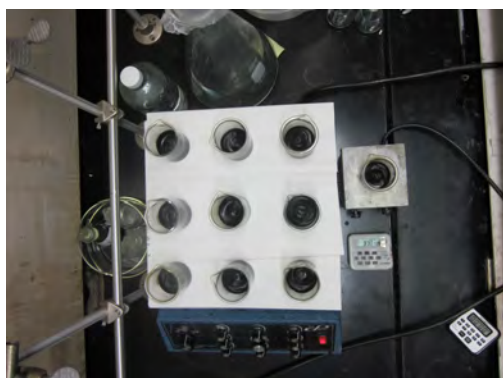
(a) Corrosion test of powder samples HJR 8B and 13B, 3:30 hours into the test with no samples displaying signs of corrosion.
