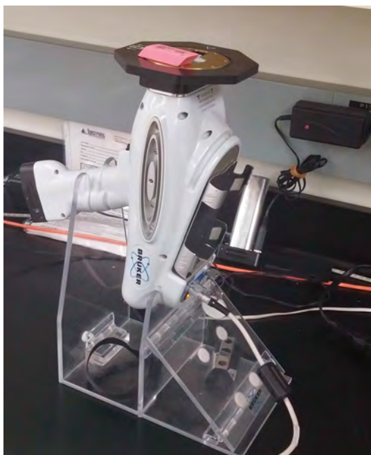
(a) Bruker Tracer III-V hand-held X-ray Fluorescence instrument resting on a stand.
