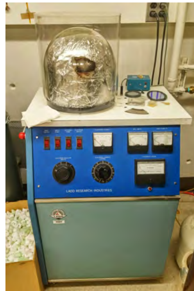
(b) Ladd carbon evaporator, used to carbon coat various samples for the SEM.
