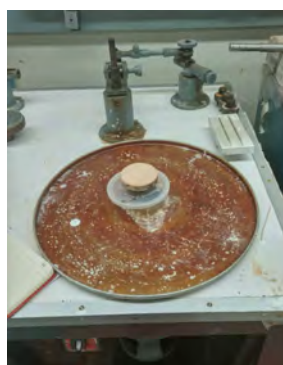
(a) The motorized grinding and polishing wheel used to polish the Stycast 1266 pucks.
