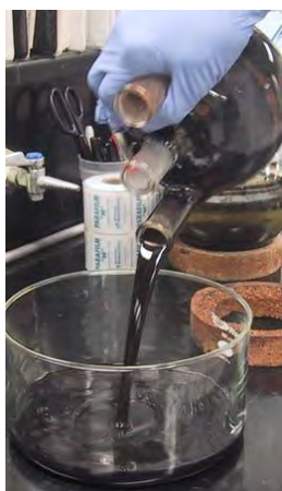
(a) The zirconium butoxide and CI-HQ slurry being poured into a crystallization dish after over-night mixing.
