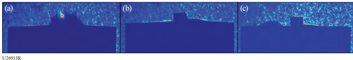
Figure 16 Shadowgraph of the target 100 ps before the main pulse arrives when a UV beam is fired (a) 3 ns, (b) 0.5 ns, and (c) 0.25 ns before the main pulse.
