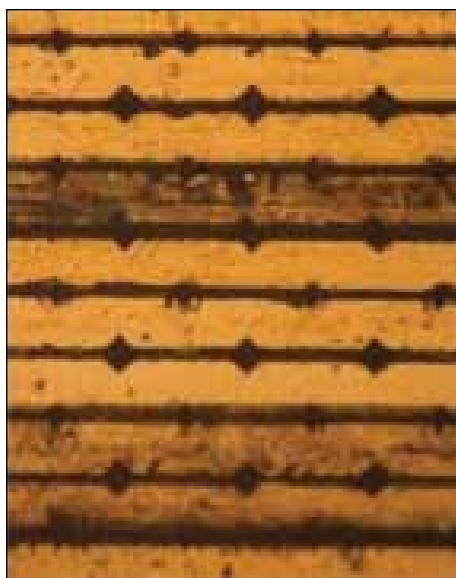
Figure 128.132 Image of the NIF Version 2 pinholes at the end of the 20-cm-long aperture body.
