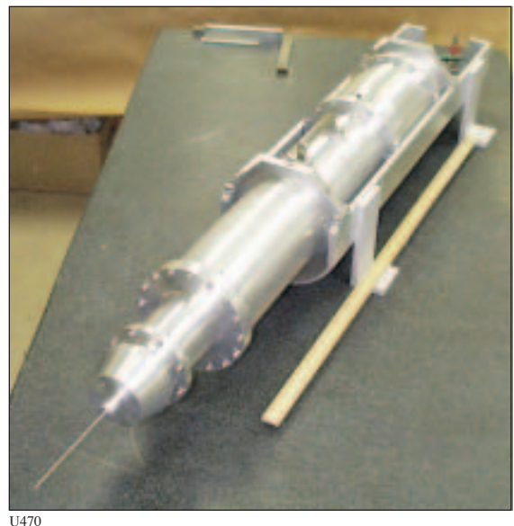
Figure 100.87 The GCD pressure cell and light-collecting optics are shown without the streak camera recording system.
