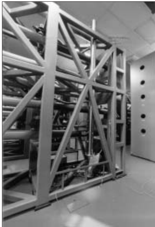
Figure 5.6-3 Spatial-filter structure with vacuum manifold riser.
