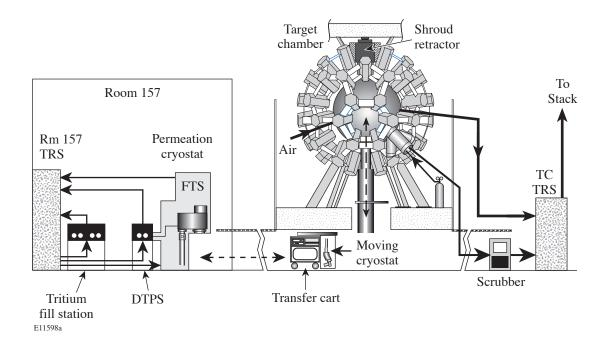
Figure 13.1-2 High-Pressure Fill Process Equipment Integration into the Tritium Recovery System.
