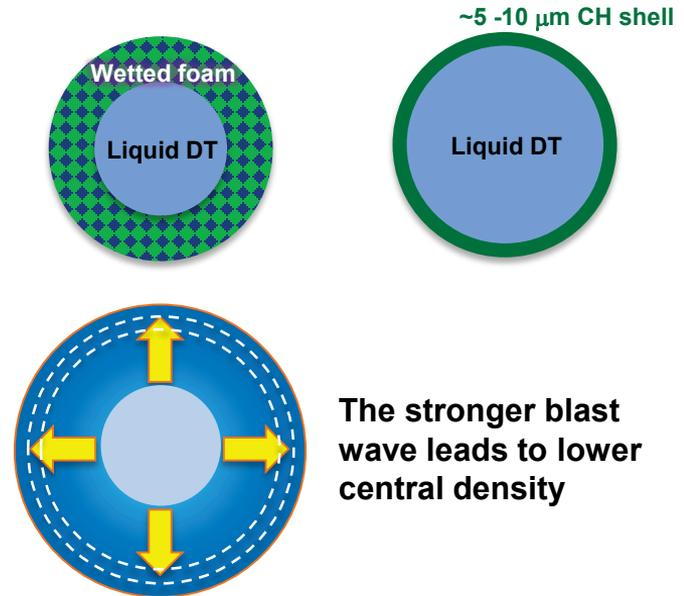
The shell and hot-spot convergence ratio can be controlled by varying central density.
