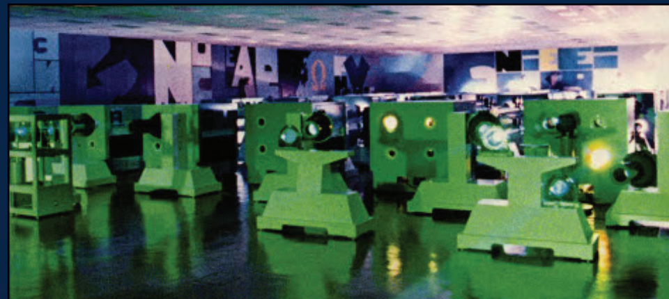
The OMEGA Laser is shown photographed in its own harmonic light. This picture was taken during system tests after the first six of the 24 infrared (1054-nm) beams were converted to 351-nm operation
