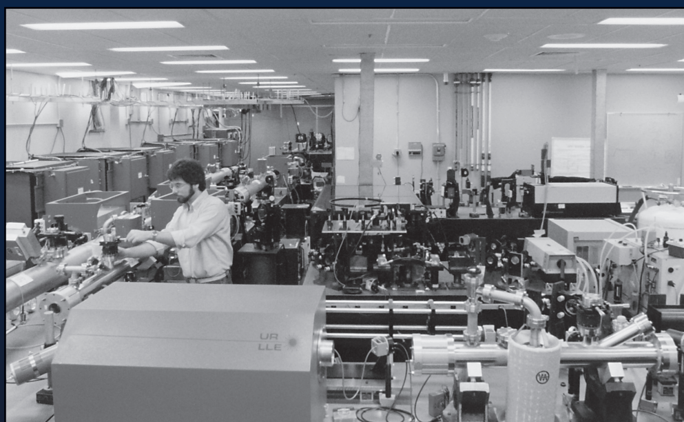
Bill Lockman, GDL operator, adjusting the pinhole of one of the vacuum spatial filters.
