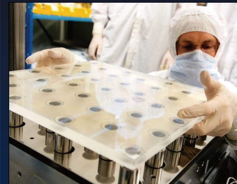
Deformable mirror being assembled by manufacturing engineer, Gary Mitchell
