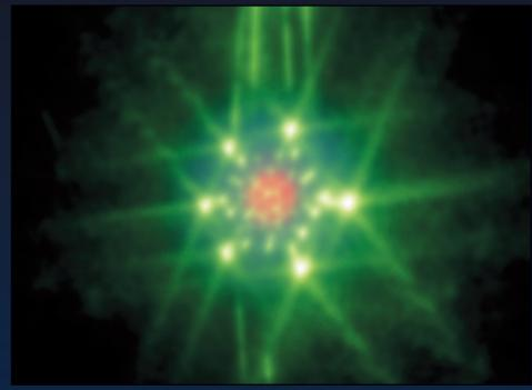
*Time-integrated photograph of an imploding OMEGA cryogenic target*
