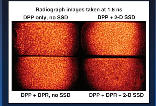
*Higher irradiation uniformity produces less imprint,* particularly with DPR's and 2-D SSD
