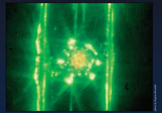
First cryogenic implosions on the 60-beam OMEGA laser showing remnants of the spider webs on either side of the imploding target
