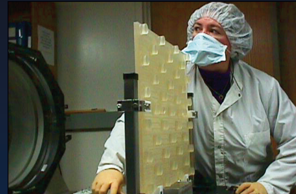
Hope D'Alessandro, electronics technician, prepares a NIF deformable mirror substrate for surface figure testing on LLE's 18-in.-aperture interferometer
