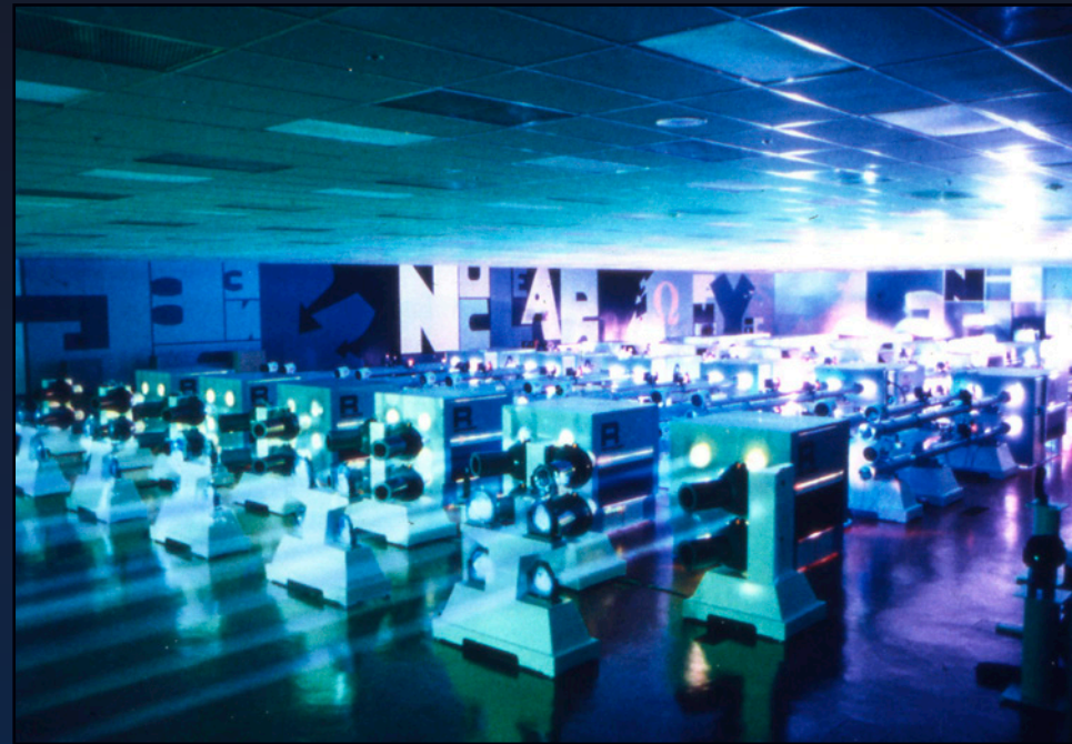
24-beam OMEGA firing, showing UV beams
