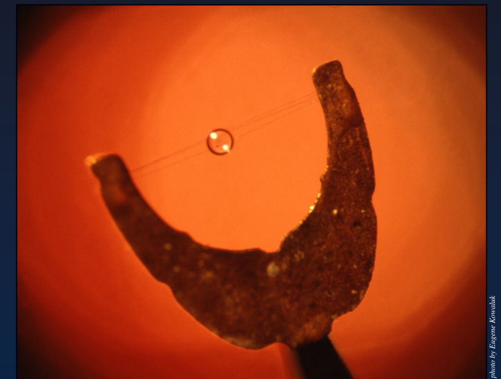
Horseshoe mount for 24-beam OMEGA cryogenic target
