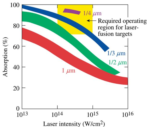
Absorption experiments at different laser wavelengths show that the energy absorbed by the capsule increases as the laser wavelength decreases. The data are obtained from several experimental facilities including LLE, LLNL, and École Polytechnique.
