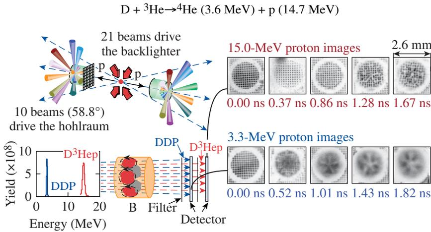
Under the NLUF program, the group from MIT led by Richard Petrasso conducted ground-breaking proton radiography experiments on OMEGA to investigate the electric and magnetic field structures inside hohlraums [143].
