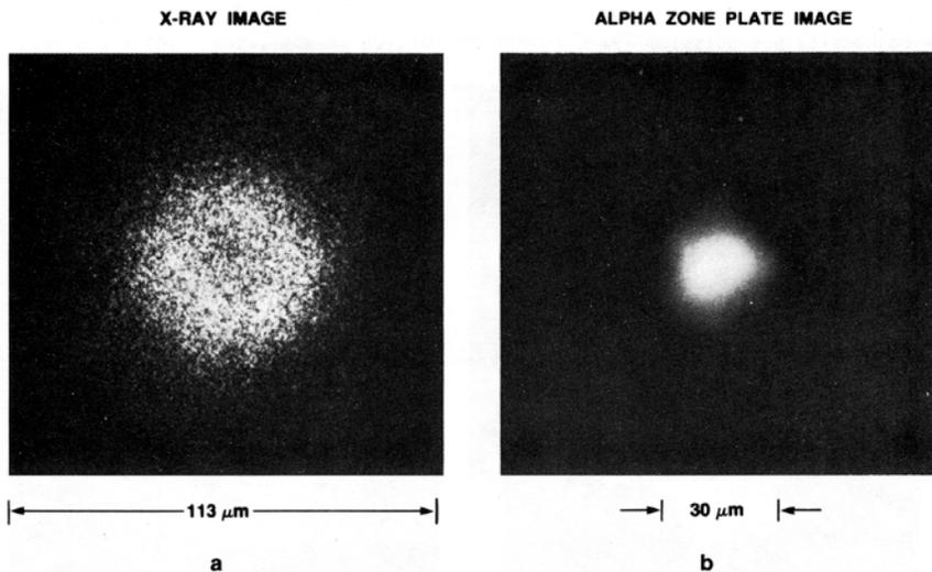
(a) X-ray pinhole camera image and (b) alpha zone plate image from an “exploding pusher”-type target shot taken on ZETA with a laser power of 1.8 TW (62-ps pulse width). The neutron yield from this DT-filled glass shell target was  $1.1 \times 10^9$  [39].
