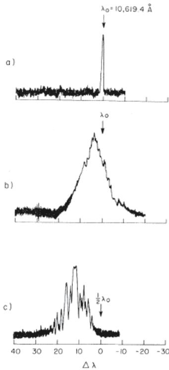
Spectral measurements made on an early laser-matter interaction experiment [6], in which single 30-J, 120-ps-wide laser pulses were used to irradiate a 150- $\mu$ m-diam LiD target: (a) incident laser light, (b) backscattered light near the fundamental frequency, and (c) backscattered light near the second-harmonic frequency.
