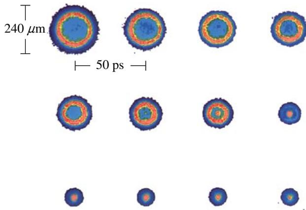
A high-speed framing camera developed at LLNL was used to image capsule implosions on the 24-beam OMEGA laser. The implosion-velocity data obtained from such experiments were used to analyze the results of the initial cryogenic capsule implosions in 1988. The first image at the upper left was taken some time after the beginning of the 700-ps-long, 1.5-kJ UV laser pulse used to implode a 240- $\mu\text{m}$ -diam, 5- $\mu\text{m}$ -thick glass shell filled with 25 atm of deuterium.
