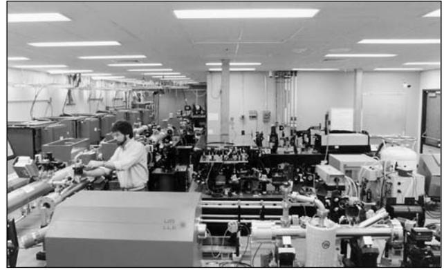
The GDL one-beam prototype laser operated for laser development and laser-matter interaction experiments at LLE from 1977 through 1993. Its major accomplishments include design validation of OMEGA; large-aperture amplifier development; the demonstration of high-efficiency frequency tripling; UV laser-matter interaction experiments; and the first NLUF experiments at LLE [26].
