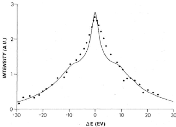
The first direct measurement of compressed density using the Stark-broadening of spectral lines. The experiment was conducted on the DELTA laser. Glass shells filled with neon gas were imploded with 40-ps, 0.2-TW pulses. The graph compares the calculated (solid curve) line profile of the Lyman- $\gamma$  of neon, at an electron density of  $7 \times 10^{22} \text{ cm}^{-3}$  to the measurements (dotted curve) [31].
