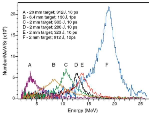
Positron spectra produced by lower-energy experiments (A–E) on the LLNL Titan laser and by an 812-J, 10-ps laser pulse on OMEGA EP (F) [147].
