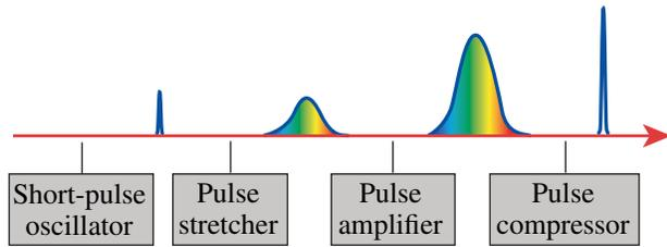
*Chirped-pulse amplification (CPA) was developed at LLE in 1985 and used to produce very high intensity ultrashort laser pulses.*
