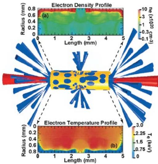
Configuration of an experiment conducted by Froula et al. (LLNL) [100] to measure laser–plasma interactions in long-scale-length NIF-like plasmas. The 5-mm-long hohlraum used in this experiment was irradiated with 51 OMEGA beams and used one the OMEGA beams as a probe: propagating down the axis of the hohlraum along a relatively uniform density plasma plateau of density  $5 \times 10^{20} \text{ cm}^{-3}$  and electron temperature  $\sim 2.5 \text{ keV}$ .
