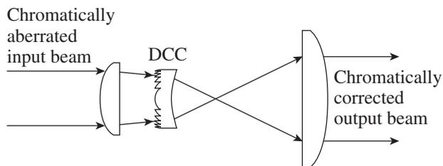
*Schematic showing the use of a diffractive color corrector (DCC) to compensate for axial chromatic aberration accumulated through the OMEGA EP Laser System. The corrector is the second element of the Keplerian telescope used to expand the OMEGA EP beam, with a diffractive lens on its flat surface.*
