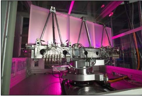
*LLE's tiled-grating assembly (TGA) is the first tiling assembly used on a petawatt-class laser system. The OMEGA EP gratings have an overall aperture of  $\sim 1.5$  m and can produce near-diffraction-limited performance.*
