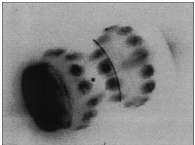
X-ray pinhole camera image of a thin-walled hohlraum implosion target [from Ref. 96] from one of the early hohlraum-drive experiments on OMEGA. The core of the imploded capsule at the center of the hohlraum is clearly seen, in addition to the joint in the hohlraum midplane made when mounting the capsule; the beam spots; and one laser-entrance hole on the left.
