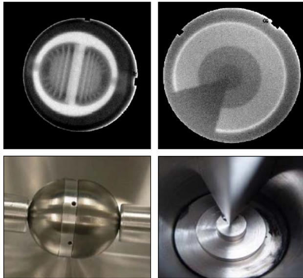
The radiography of massive objects with high-resolution MeV-photon imaging was demonstrated by a collaborative team led by CEA in 2010 OMEGA EP experiments. On the left are the test objects named "flower" (bottom) and its radiographic image (top); on the right are a step-wedge object named the "tower of Hanoi" (bottom) and the resulting radiography image (top). These images were produced using a single OMEGA EP beam operating at  $\sim 1$  kJ in  $<10$  ps.
