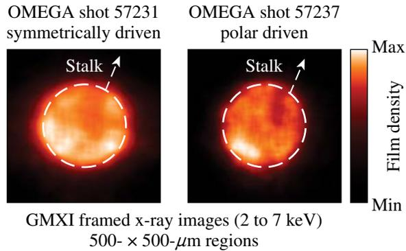
Film-recorded framed x-ray images of implosions of DT-filled glass targets obtained with the GMXI framed x-ray imager near the time of stagnation for both a symmetrically driven target (left) and a polar-driven target (right). The target stalk direction is indicated by the dashed arrows.
