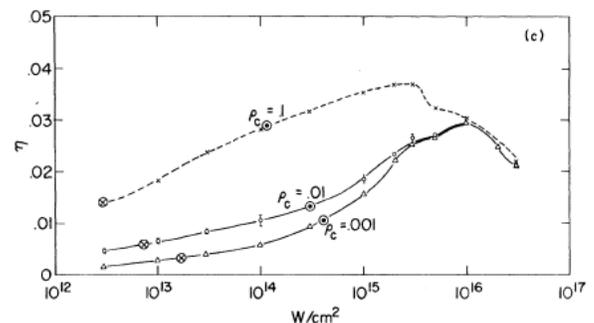
Plot from the McCrory and Morse paper of 1977 [25] showing the predicted dependence of hydrodynamic efficiency on the laser intensity for different values of critical density. The paper concluded that the hydrodynamic efficiency in laser-driven implosions would increase by a factor of 3 to 5 if the laser wavelength was reduced from the infrared to the ultraviolet.
