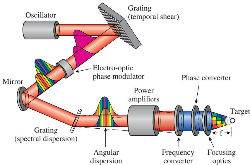
*Schematic illustrating the SSD concept.*
