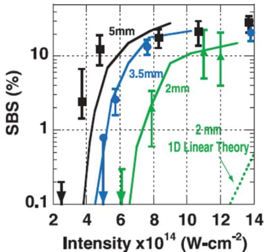
Stimulated Brillouin scattering (SBS) results from the long-hohlraum experiment showing the percentage of SBS as a function of beam intensity for several different plasma lengths. The solid curves are predictions obtained from the SLIP code. For reference, a curve (dashed) is shown that was calculated using linear theory for the 2-mm-long case where an SBS gain of  $\sim 11$ , for an intensity of  $1 \times 10^{15} \text{ W/cm}^2$ , is determined by postprocessing the hydrodynamic properties.
