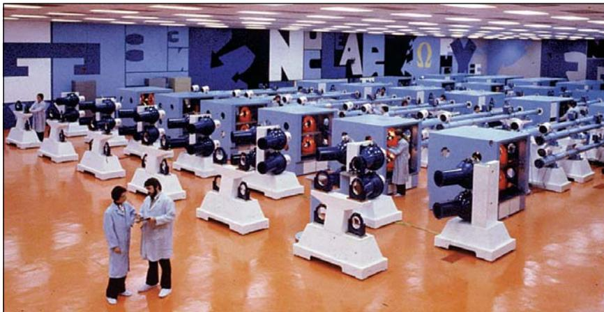
View of the 24-beam OMEGA laser.
