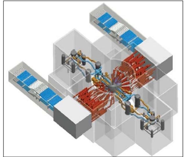
*Conceptual designs of inertial fusion power plants based on laser drivers have been developed over the last few decades [176]. The laser for one such design from LLNL (shown above) is based on diode-pumped glass.*
