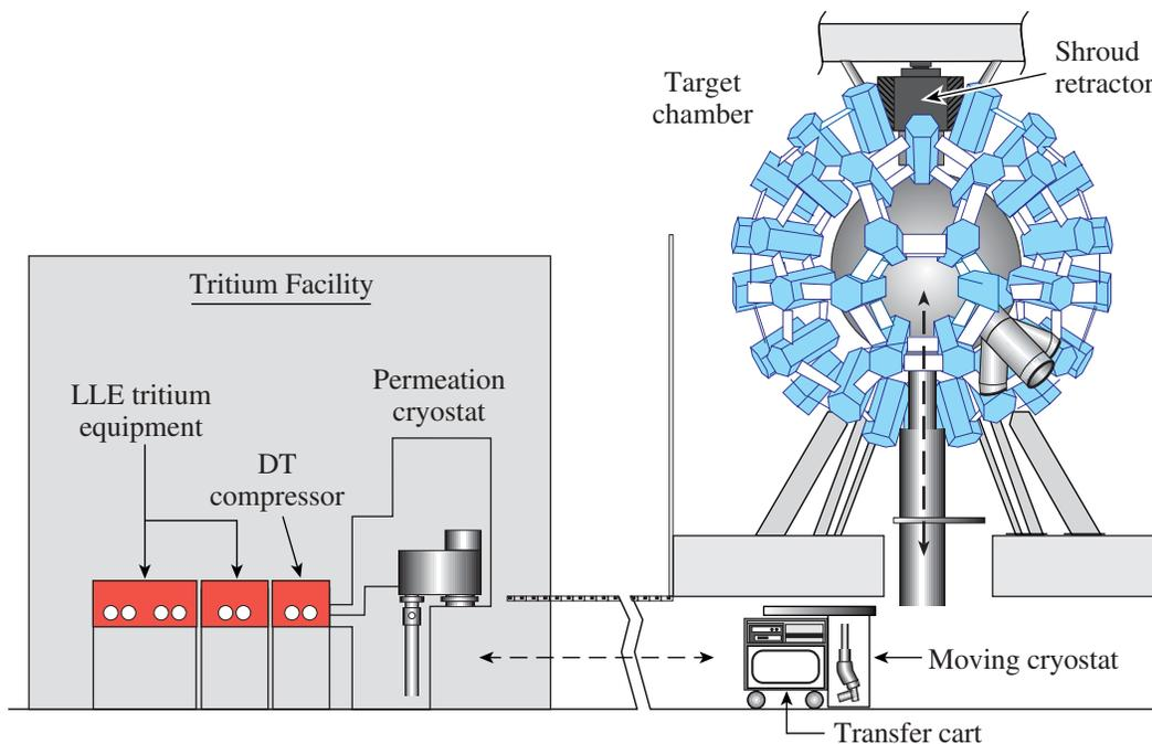
Schematic of the OMEGA Cryogenic Target Handling System.
