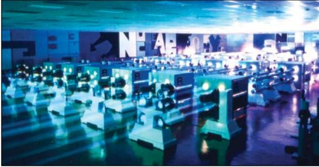
*Stephen Craxton (left) and Wolf Seka (right) led the LLE effort to develop an efficient frequency-conversion scheme. The full 24-beam OMEGA laser was frequency converted to the ultraviolet in 1985 (bottom).*
