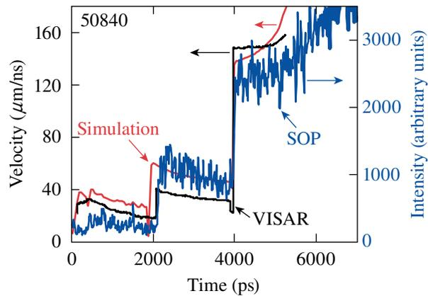
Key to the achievement of OMEGA high-density implosions as well as the demonstration of ignition on the NIF is the precise measurement and control of timing of the shocks that coalesce to form the high-density core of an imploding capsule. This figure shows measurements of the shock velocity and timing of multiple shocks in a liquid-deuterium target performed using the VISAR (black curve) and SOP (blue curve) diagnostics on OMEGA compared to hydrodynamic code simulations (red curve) [120].
