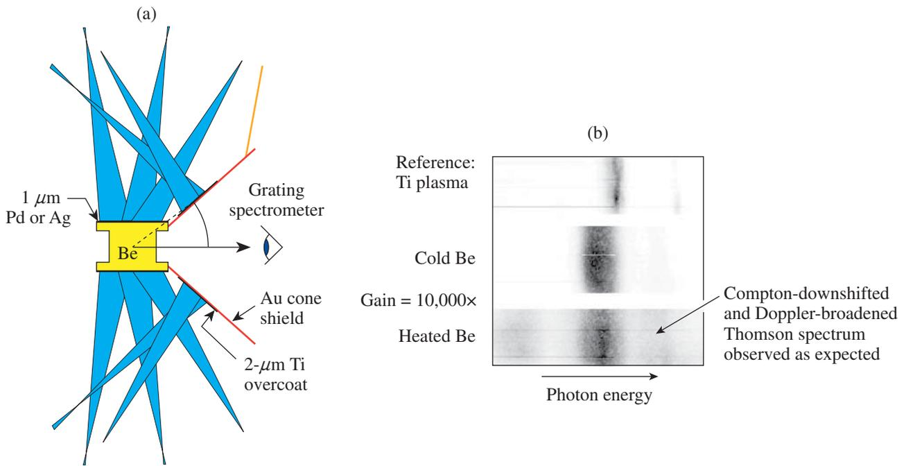
An important diagnostic development on OMEGA occurred when LLNL scientists [99] demonstrated, for the first time, x-ray Thomson scattering as a temperature and density diagnostic for dense plasma.
