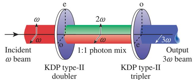
Schematic illustration of Craxton’s frequency-tripling scheme.
