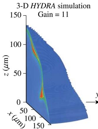
*2-D (left) and 3-D (right) simulations of NIF polar-drive capsules show that ignition and gains of 17 and 11, respectively, are predicted for polar drive at a NIF energy of ~1 MJ.*
