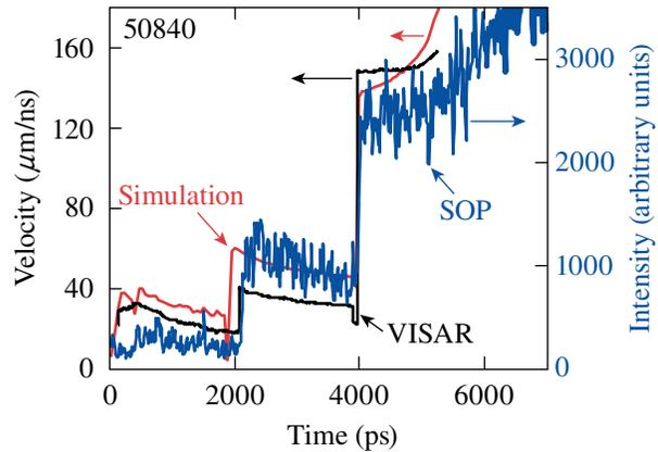
Key to the achievement of OMEGA high-density implosions as well as the demonstration of ignition on the NIF is the precise measurement and control of timing of the shocks that coalesce to form the high-density core of an imploding capsule. This figure shows measurements of the shock velocity and timing of multiple shocks in a liquid-deuterium target performed using the VISAR (black curve) and SOP (blue curve) diagnostics on OMEGA compared to hydrodynamic code simulations (red curve) [120].
