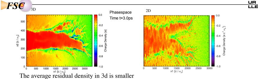
$V_{3D}$  =2  $V_{2D}$  due to stronger laser selffocusing and easier channeling in 3D
