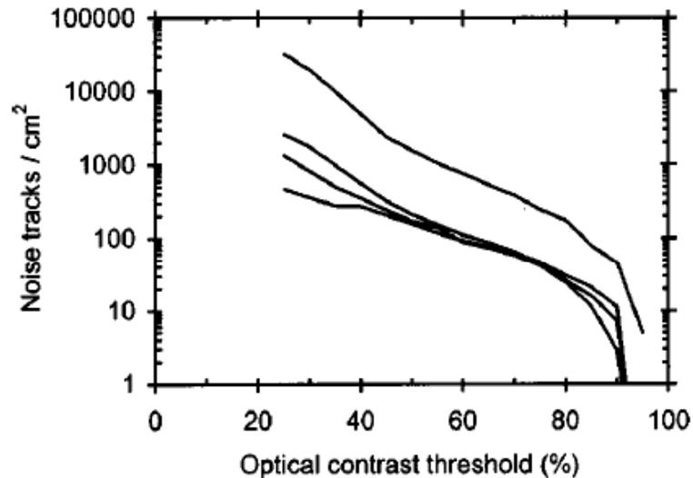
The lower limit of neutron yield detection occurs when the intrinsic noise and the neutron track densities are of the same order
