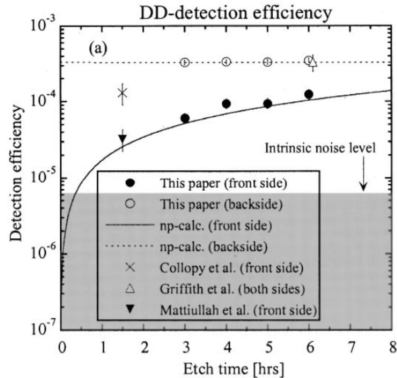
The total efficiency must take into account the neutron detection efficiency of CR-39 as well as the proton detection efficiency at various angles of incidence.
