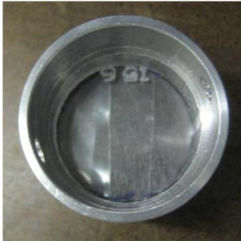
CR-39, on top of CH<sub>2</sub> (layered from left to right: 100, 50um, 0um) on top of 1mm of tantalum
