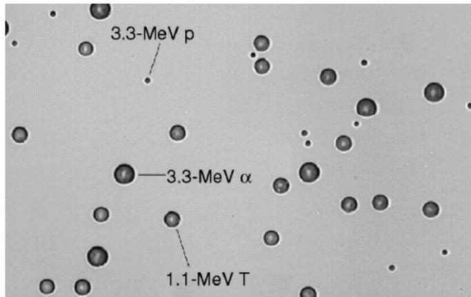
CR-39 is etched after exposure to reveal charged particle tracks. Track size is proportional to the stopping power of charged particles,  $dE/dx$  as well as the etch time
