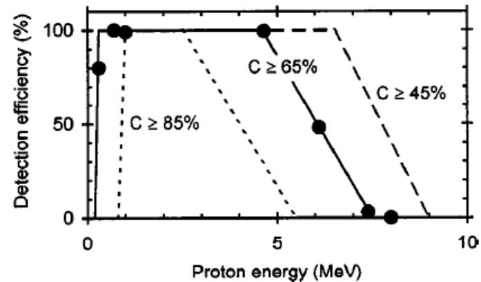
CR-39 has a 100% detection efficiency for protons up to 5MeV at normal incidence. Contrast limits on track diameters may be imposed during analysis; efficiency for several user selected contrast values are shown
