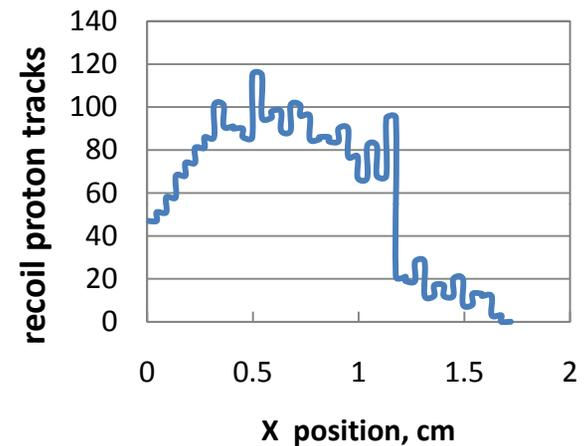
Analysis of scanned detector piece, again showing the corresponding step in number of detected tracks going from 50um to 0um of CH<sub>2</sub>
