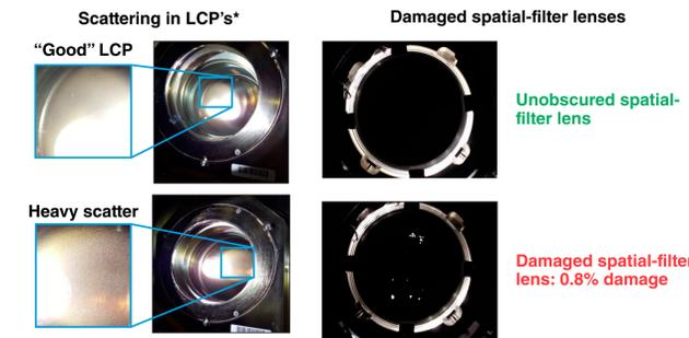
Transmission losses of up to 3% were addressed.
