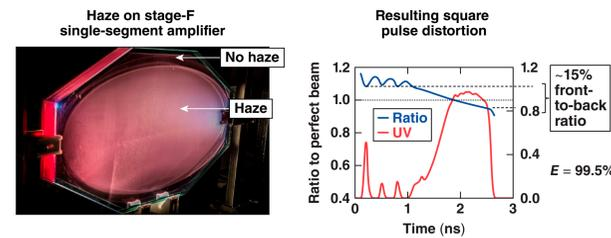
Rough guide: 1% unbalanced loss results in 2% pulse tilt.
