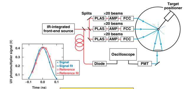
Beam timing is maintained to <5 ps.
