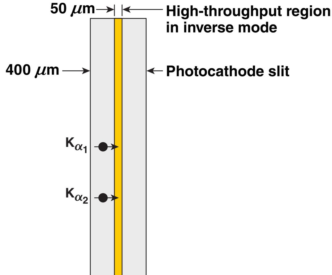
The alignment plate is the crucial component for transferring alignment from an x-ray CCD to the photocathode.
