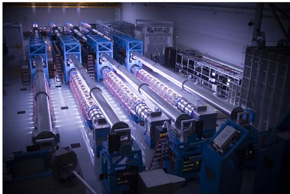
OMEGA EP Laser System: 2.6 kJ, 10 ps
