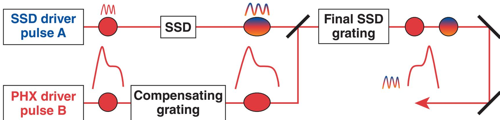
**SSD bandwidth is only applied to one pulse to generate dynamic bandwidth reduction.**
