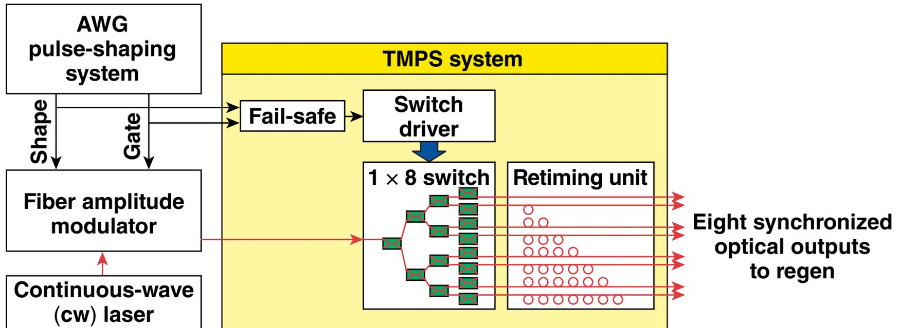
**TMPS minimizes interpulse jitter for two co-propagating drivers.**
