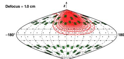
The contours are more spread out for a defocused beam
