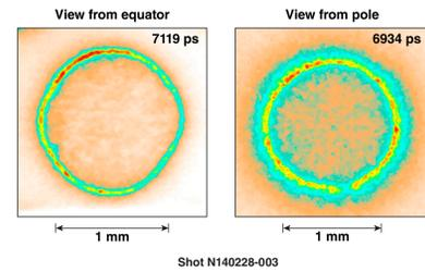
Azimuthal variations around  $\theta = 60^\circ$  are reduced by a factor of 2 using the defocused design
