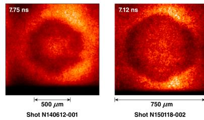
The energy deposition pattern for a single beam shows closely spaced contours
