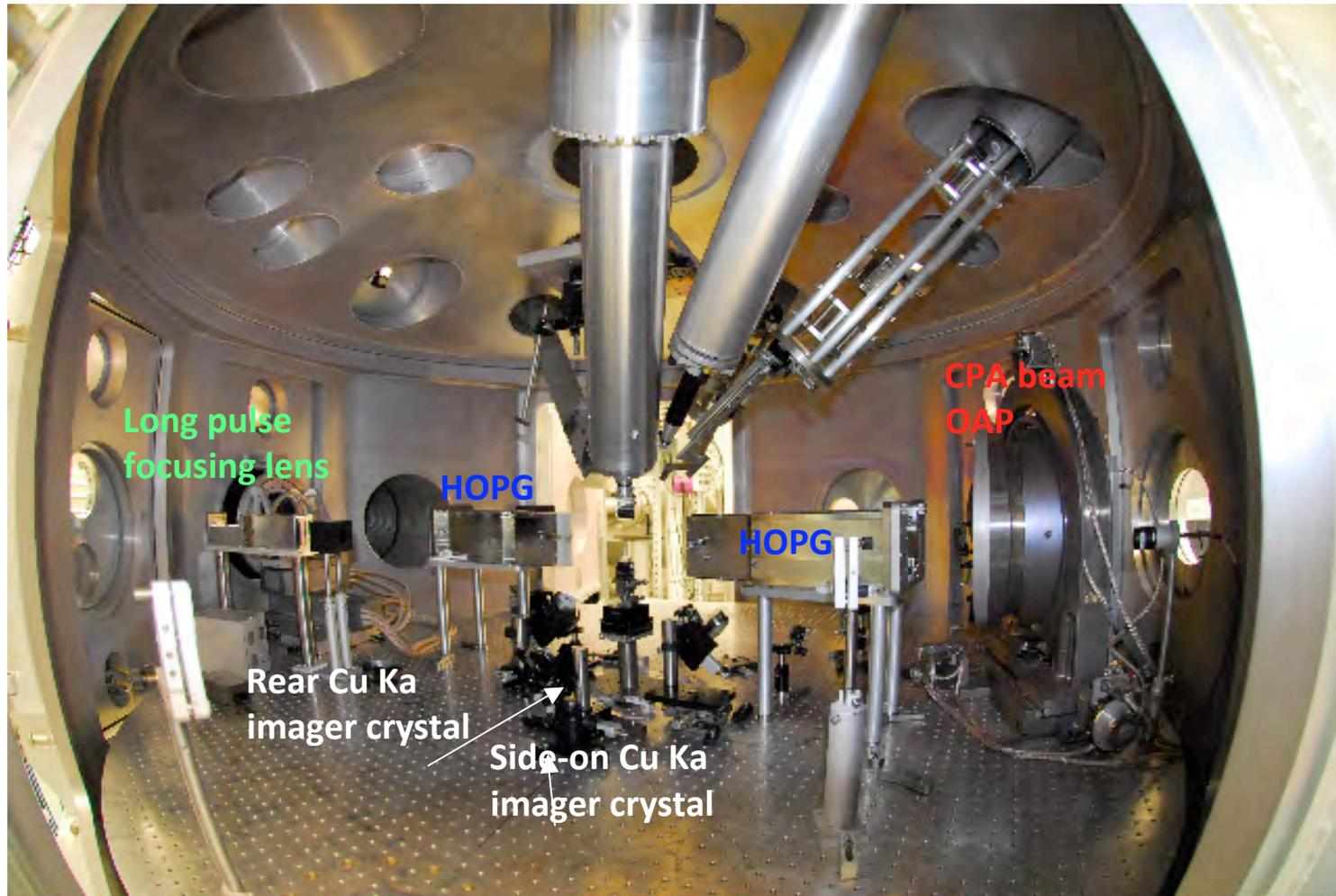
A comprehensive diagnostics suite was used to characterize transport properties by measuring **Cu K $\alpha$  yields and spatial profile** as well as **fast electron spectrum**
