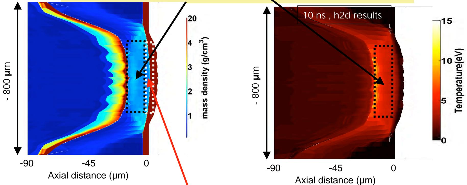
Fast electrons transport across the density gradient at the Au/WDM interface
