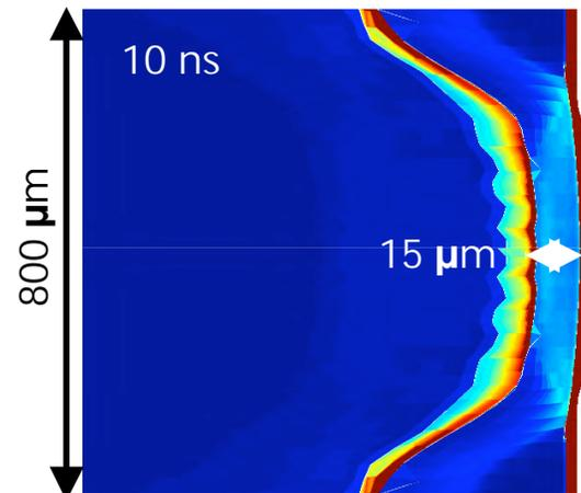
Cu K $\alpha$  imager revealed critical information of fast electron angular distribution in WDM transport exp.
