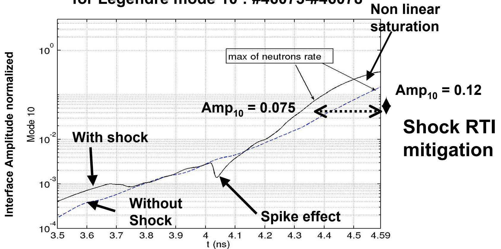
Although the RTI growth rate with spike is greater at the maximum of neutrons rate, the interface D<sub>2</sub>-CH amplitude is smaller.
