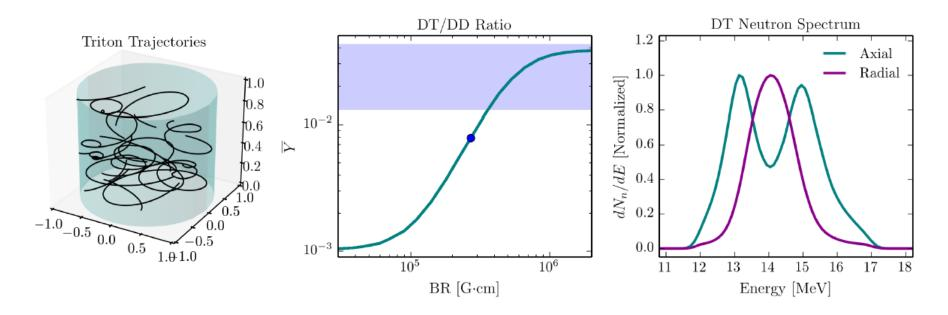
The pre-imposed  $B_z$  field magnetizes the plasma trap the tritons and direct them axially in helical orbits.
