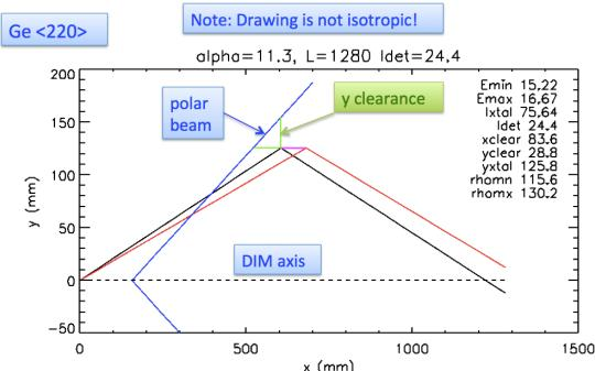
Determine pattern of rays hitting photocathode as function of where they hit crystal
