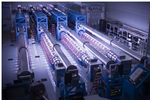
OMEGA EP Laser System: 2.6 kJ, 10 ps Frequency: 1\omega Intensity: >10^{18} W/cm 2
