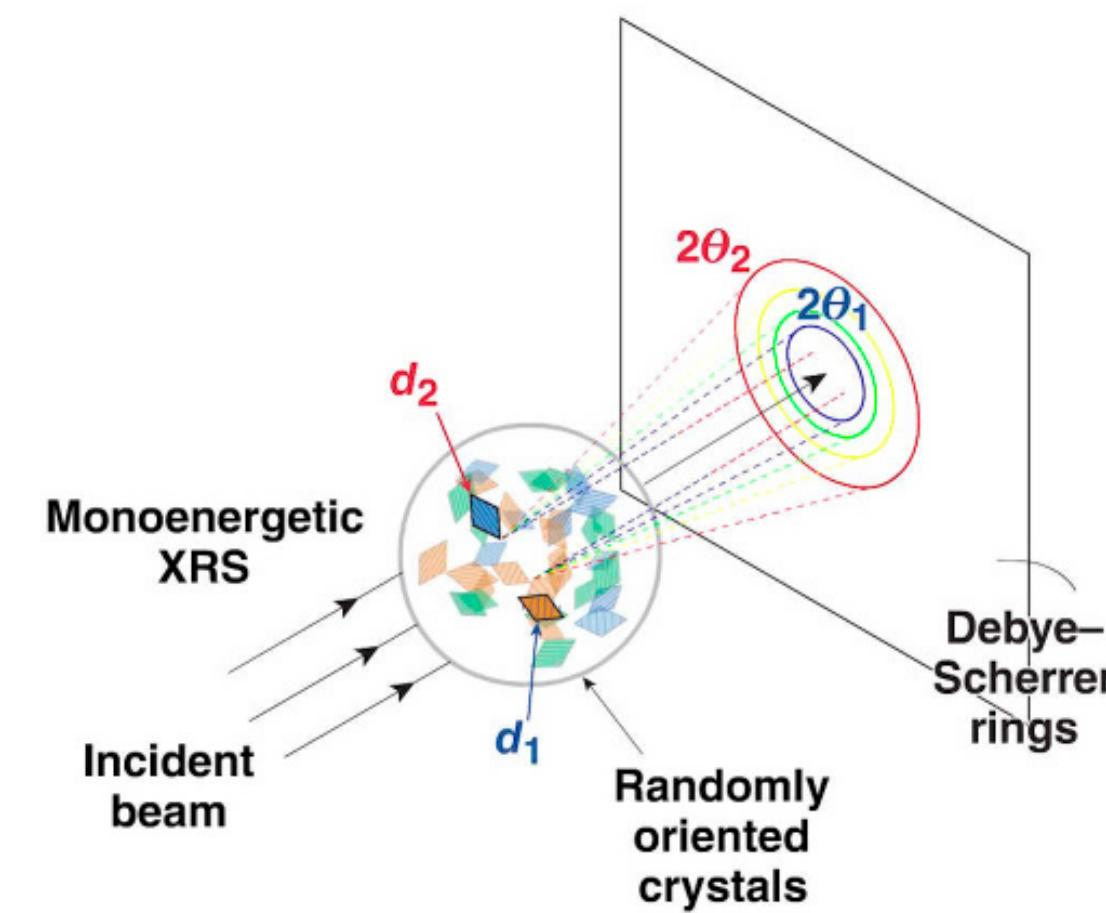
Compression of interatomic spacing ( $d$  spacing) is determined by measuring diffraction angles ( $2\theta$ ) and x-ray wavelength ( $\lambda$ ).
