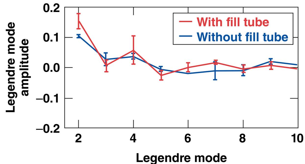
The fill tube slightly increases the amplitude of the  $\ell = 2$  mode.
