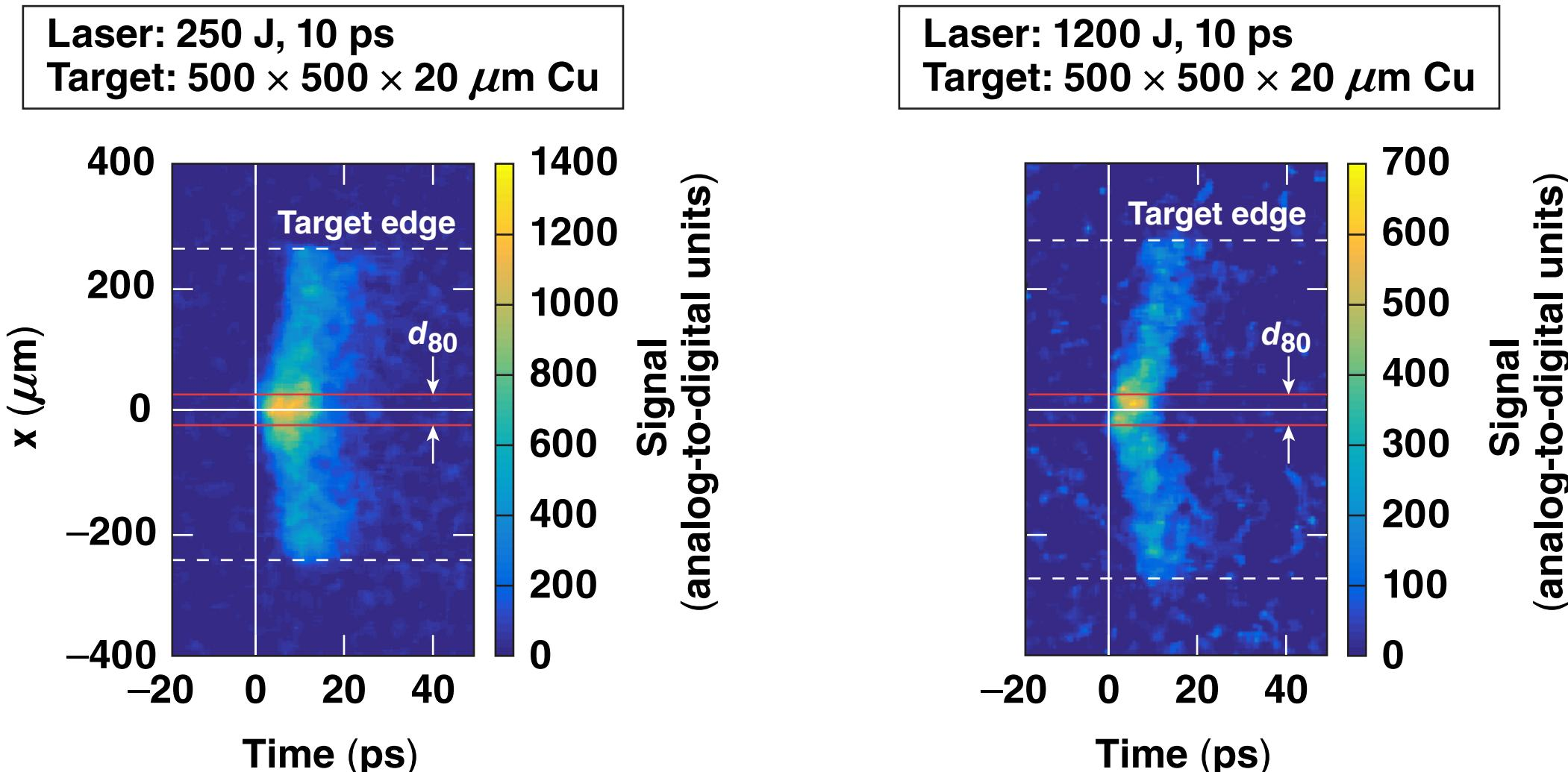
The initial hot-electron beam diameter is comparable to the laser focal-spot size.
