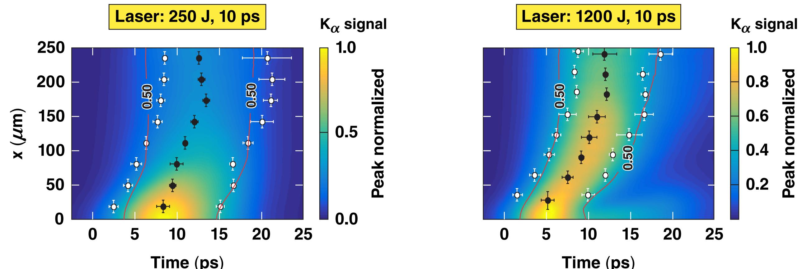
Target heating suppresses  $K_{\alpha}$  emission from the central regions of the target.
