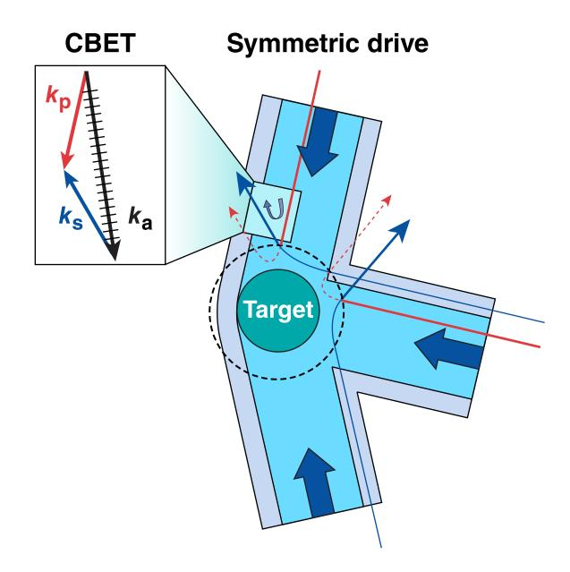
Simulations indicate that CBET reduces the ablation pressure by up to 40% in symmetric-direct-drive implosions on OMEGA.\*
