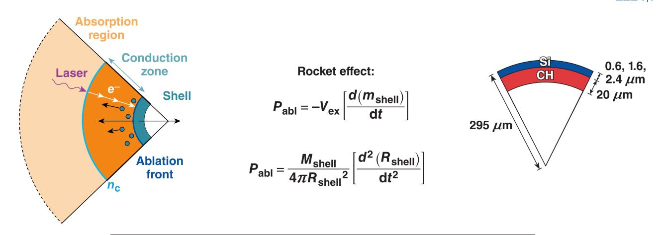
Simultaneous measurements of the mass ablation rate and shell velocity constrain the hydrodynamic coupling.
