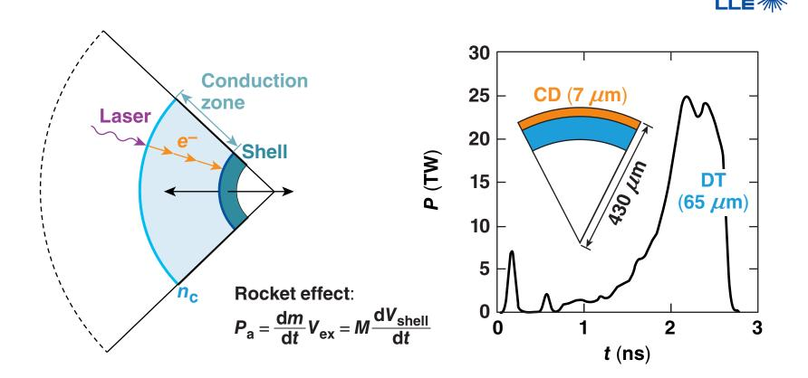
Measurements of the trajectory ( $V_{shell}$ ) and the CD burnthrough [(dm/dt), M] constrain the coupling physics in direct-drive implosions.
