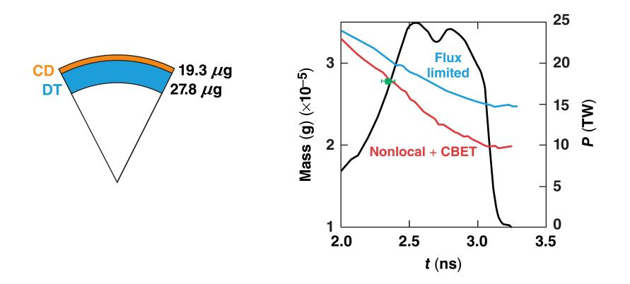
When matching shell trajectory, time-dependent flux-limiter simulations overestimate the shell mass and the kinetic energy by 26%.
