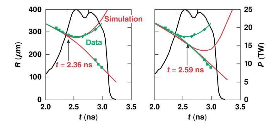
When matching shell trajectory, time-dependent flux-limiter simulations predict a burnthrough time 250 ps later than in the experiment.
